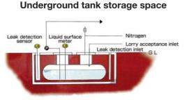
Making underground tanks double-layered (Kagoshima Sendai Plant) Underground tanks are placed in concrete rooms and this structure helps the early discovery of leakage and prevents further leakage.
