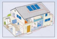
Schematic Diagram of a Solar Water-Heating System
