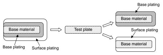
Prepare the test plate by using such as SUS304, and measure the weight.
