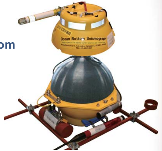
The Self-Surfacing Ocean-Bottom Seismograph is an instrument designed to measure and record earthquakes on the ocean floor. After measurement, the main body floats to the surface and is recovered by a ship. Earthquake data is then analyzed.
